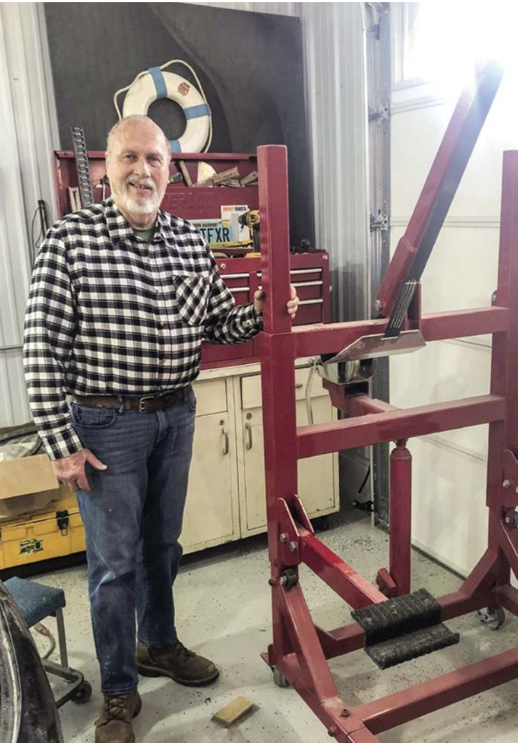
Bob Gibbons poses with a smaller version of his original capsizer. This model is used to repair small watercraft, such as Jet Skis and WaveRunners.
