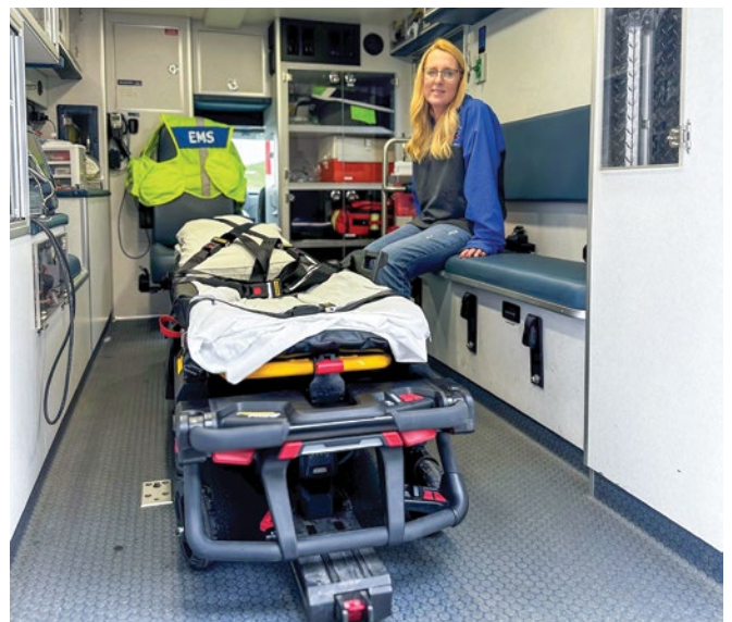
LeeAnn demonstrates the power cot once it is anchored in place inside the ambulance.
